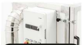
Control Board PLC
